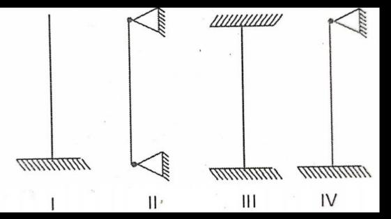
It is required to order these four beams in the increasing order of their respective first bucking loads. The correct order is given by A : I, II, III, IV B : III, IV, II, I C : II, I, IV, III
